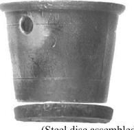
Internal diameter at top: 42mm (1 21/32") External diameter to edge of flange: 49mm (1 15/16")
