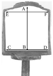
The A-B measurement= Maximum internal height
