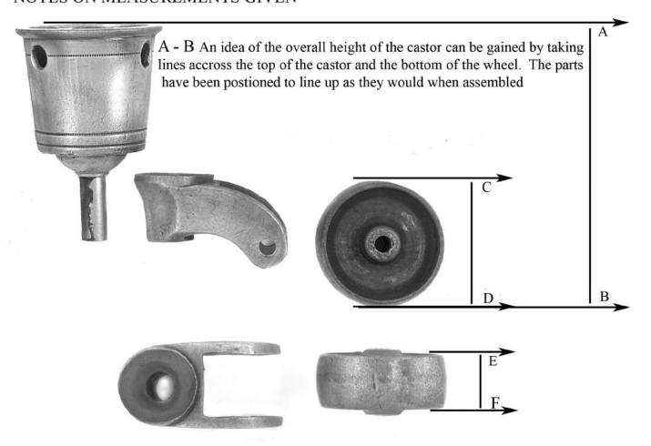
C - D Wheel diameters have been measured on the crown of the wheel.
